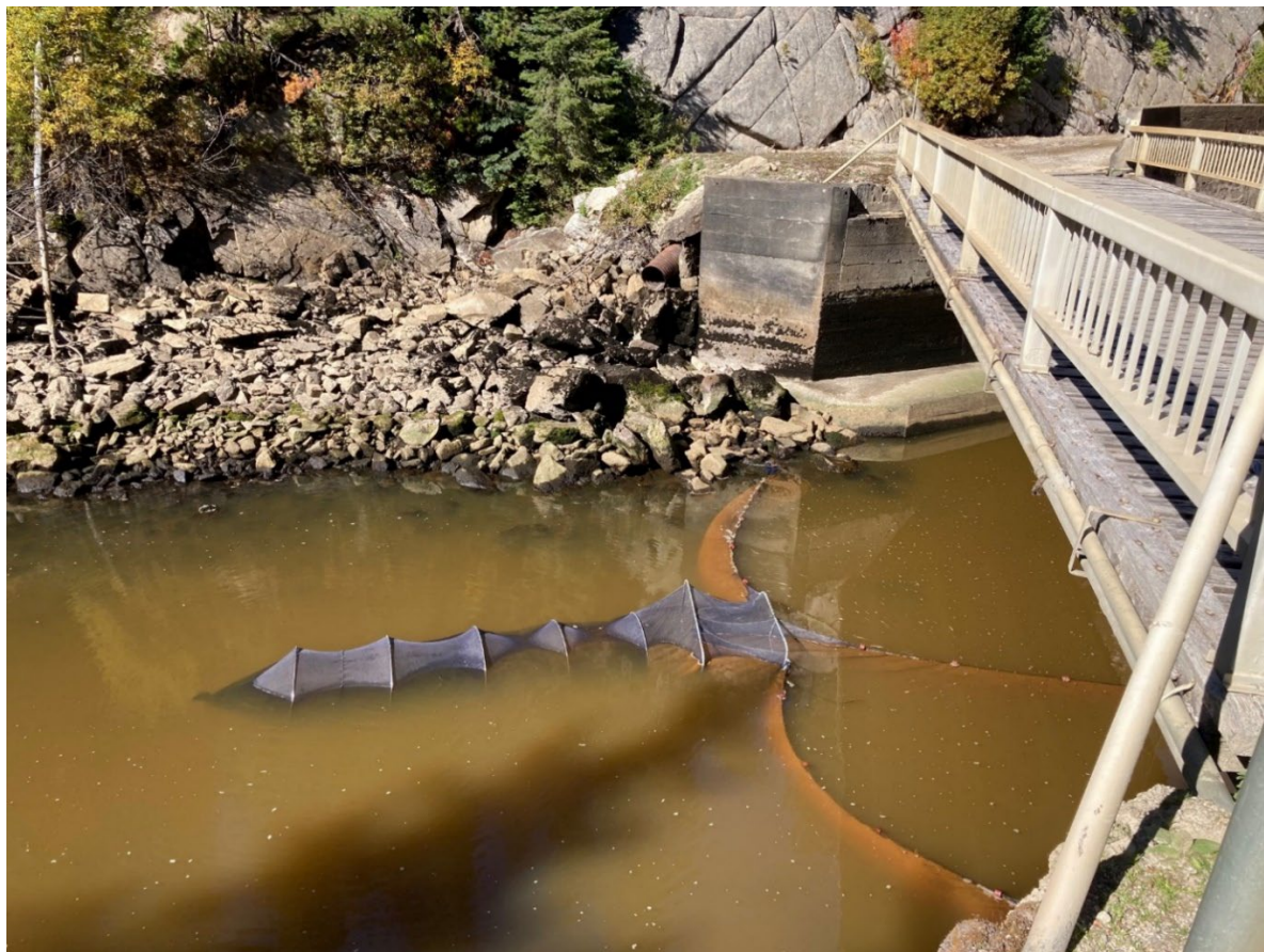
Figure 12. Fyke net location under the access bridge to the dam. Wings were attached to both shorelines and lead line was angled around bridge abutment and anchored to the river left shoreline. This location worked well and should be used in the future. Note that algae, detritus, and oxidized iron sediment accumulated on wings. Fish were generally loaded/unloaded on the concrete shelf under the bridge.
